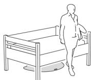
If call triggering is not necessary, place the pressure mat where it cannot be walked on.
